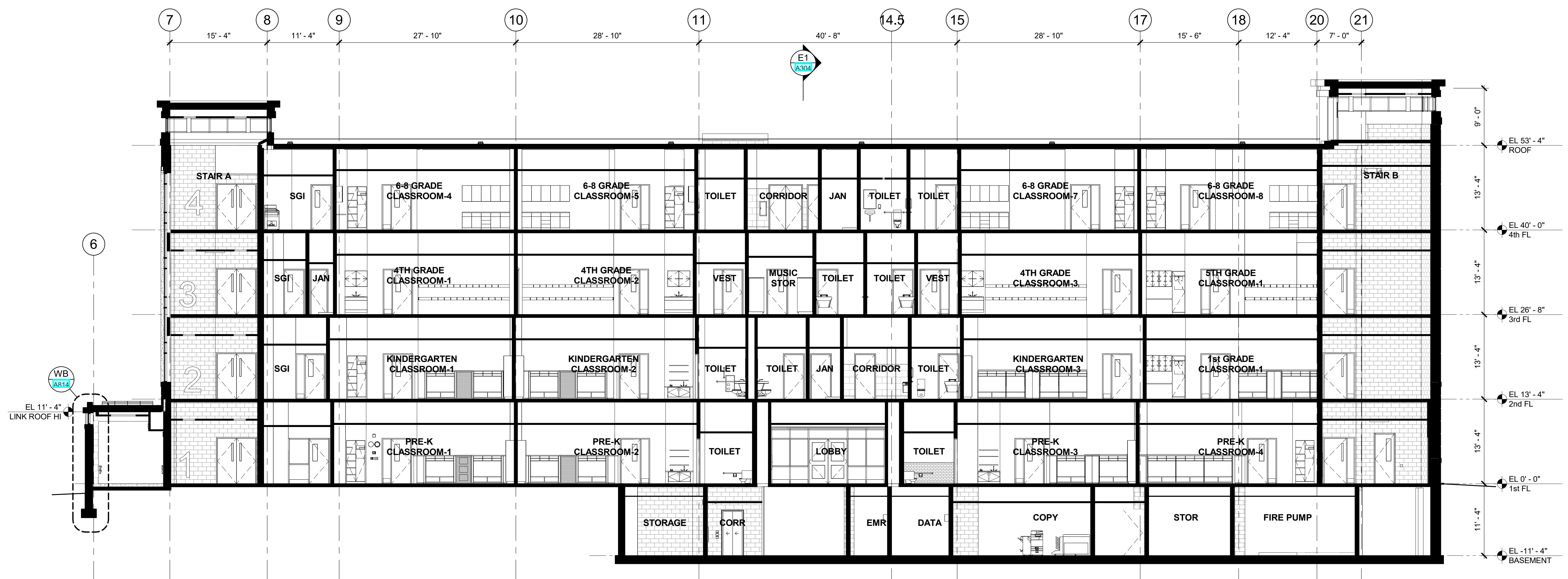
N1 BUILDING SECTION N1 - LOOKING NORTH1 1/8" = 1'-0"
