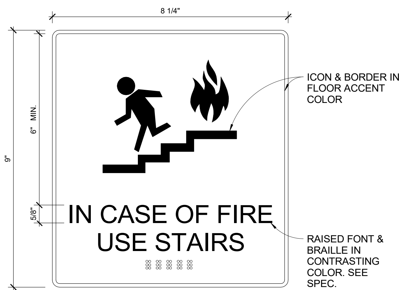
TYPE F ELEVATOR SECONDARY SIGN
