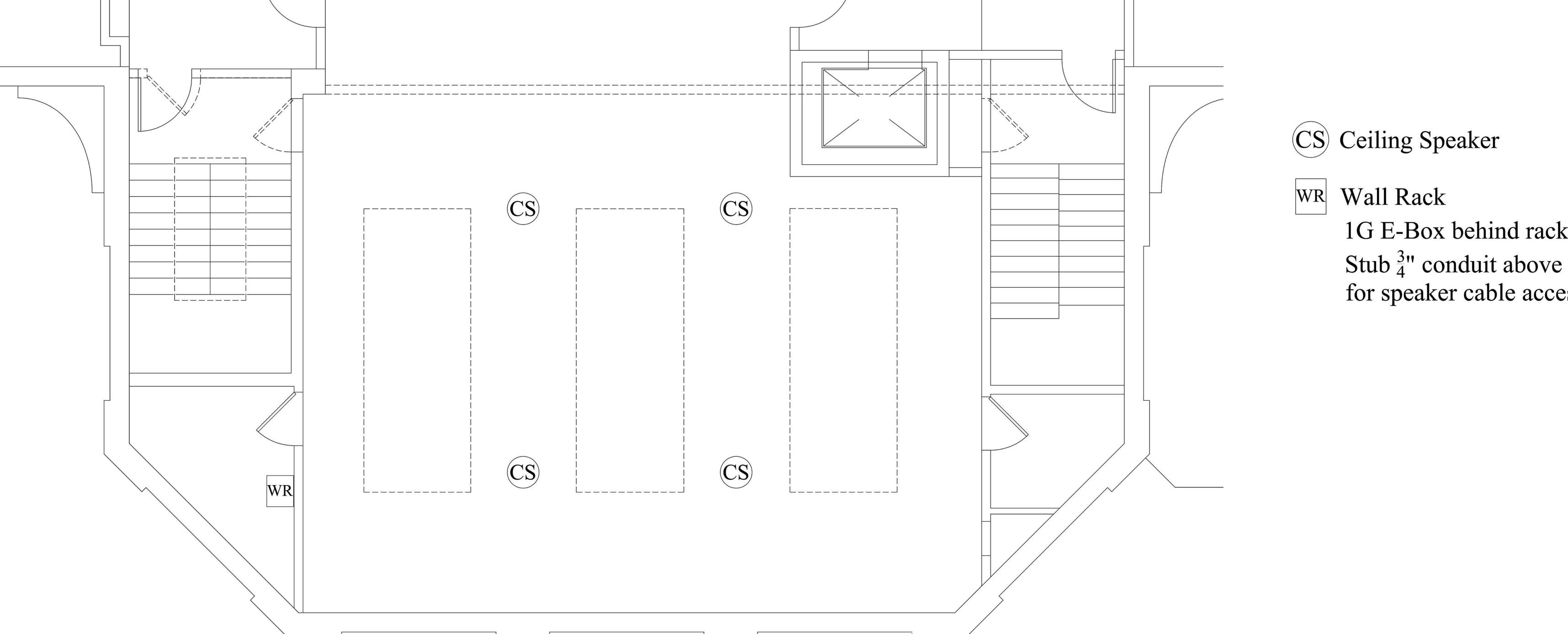
1G E-Box behind rack, Stub  $\frac{3}{4}$ " conduit above ceiling for speaker cable access.
