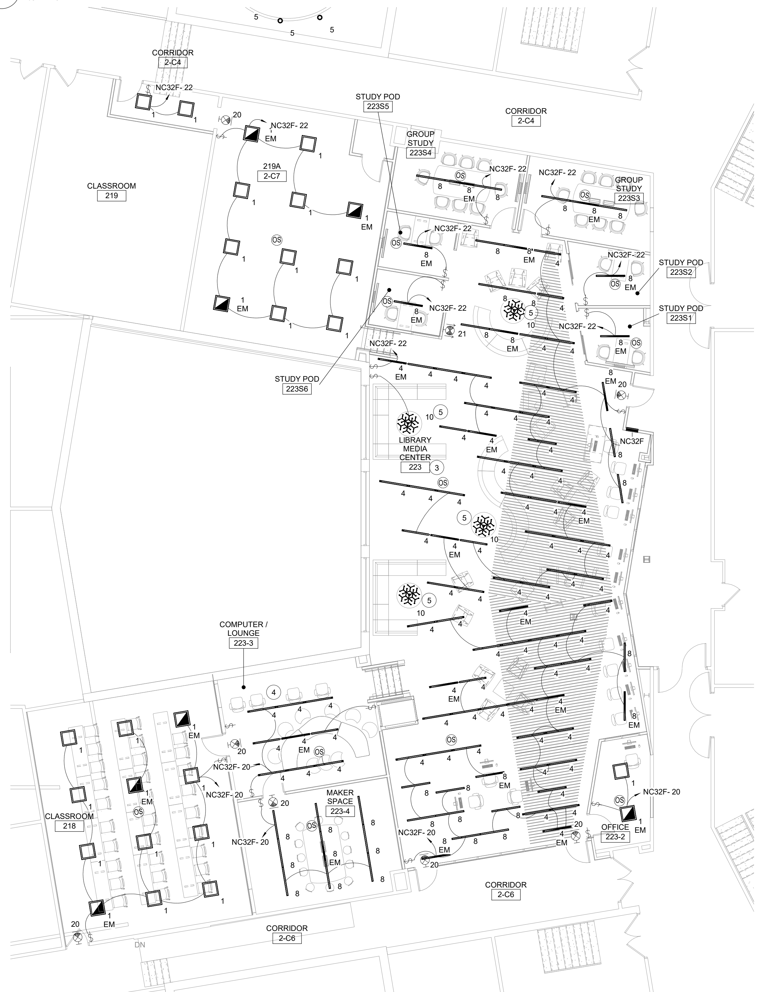
4 2nd Floor - LMC Lighting Plan - Area C 1/8" = 1'-0"
