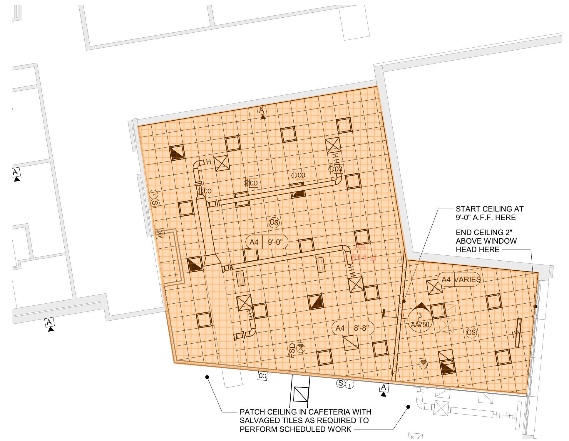
2 Basement - Cafeteria & Kitchen - Reflected Ceiling Plan 1/8" = 1'-0"
