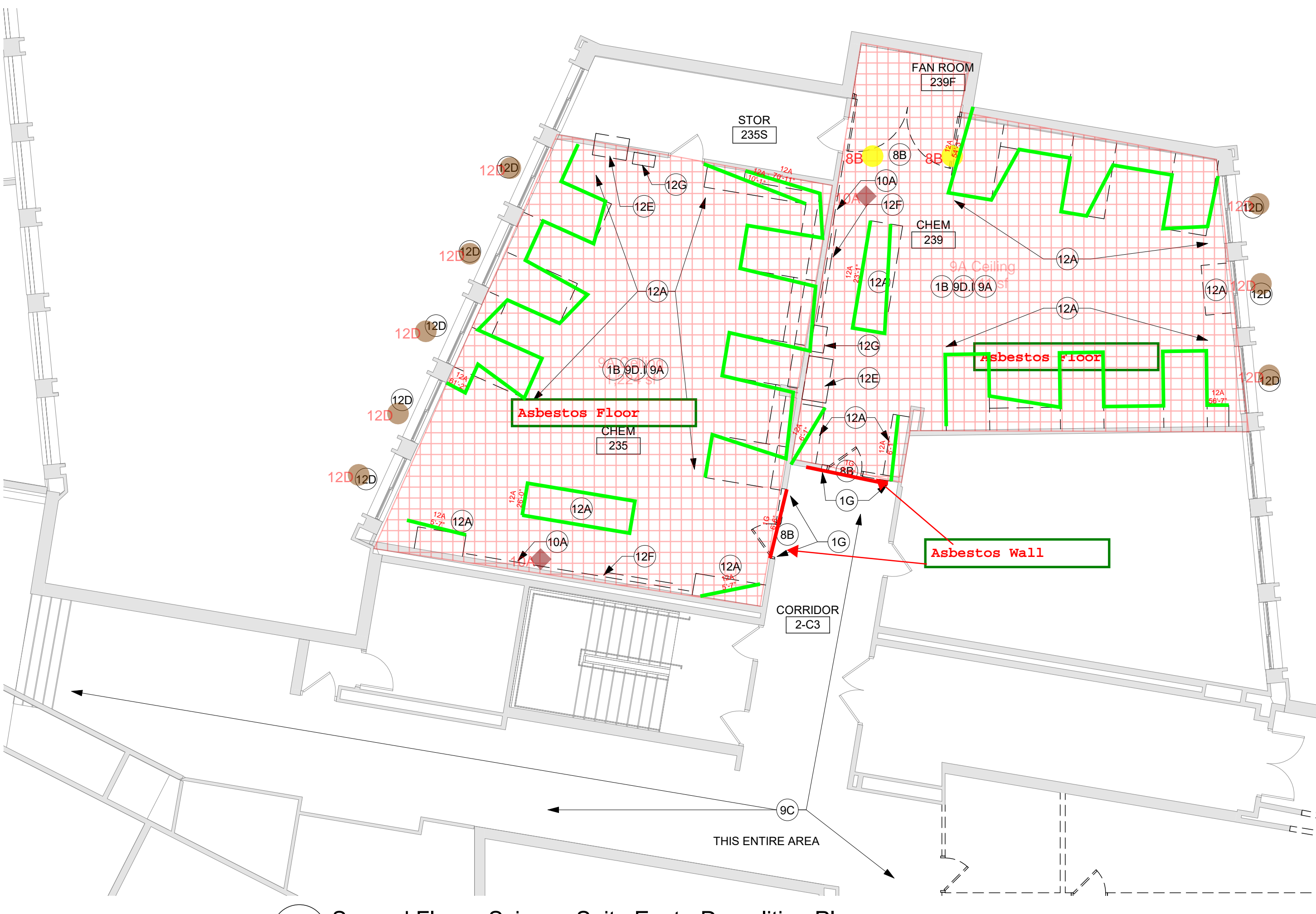
2 Second Floor - Science Suite East - Demolition Plan 1/8" = 1'-0"
