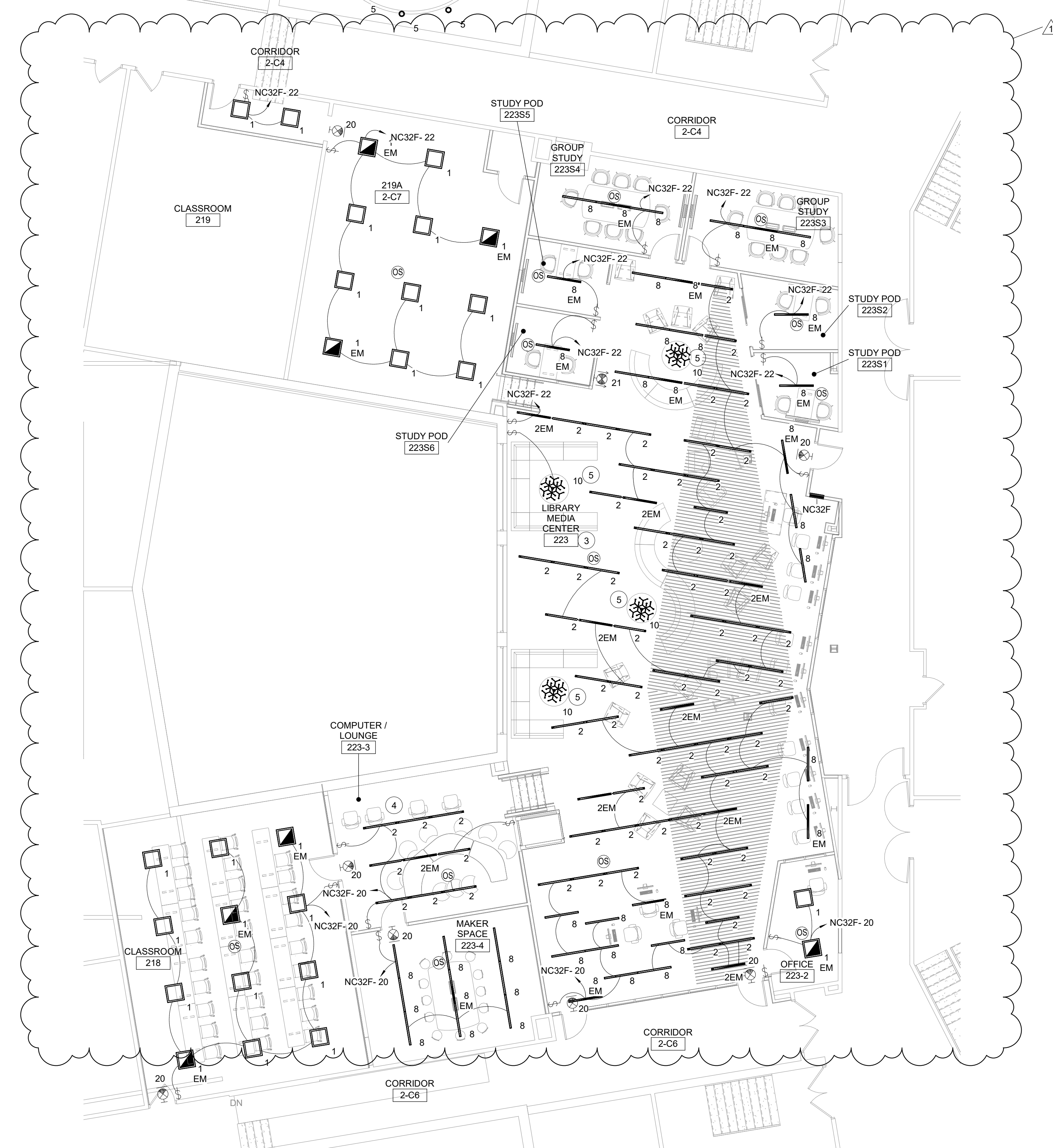
4 2nd Floor - LMC Lighting Plan - Area C 1/8" = 1'-0"
