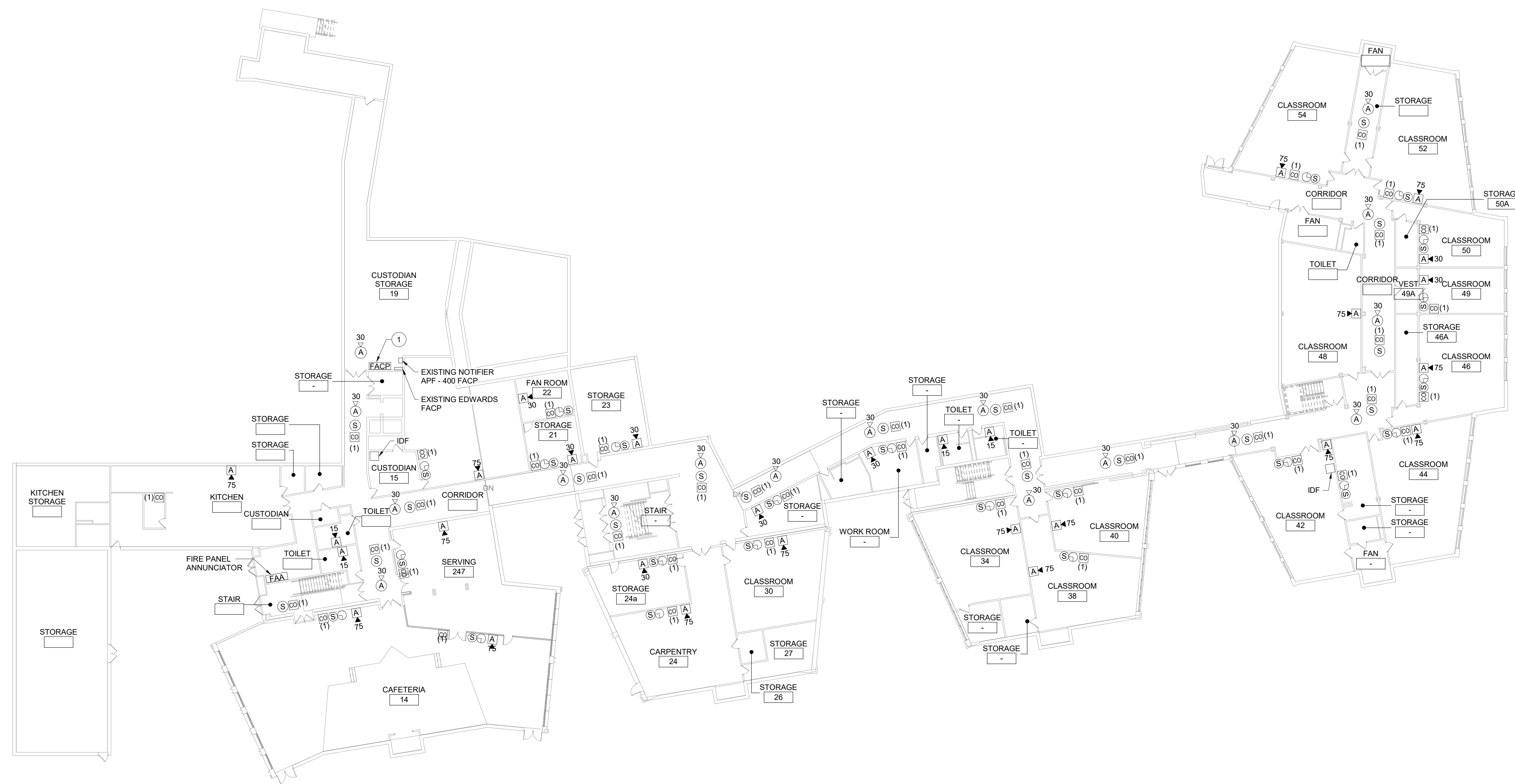
1 Basement Speaker, Clock and Fire Alarm Plan - Areas B, C, D & E 1" = 20'-0"
