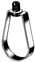
C-727/CT-727 Adj. Swivel Ring Hanger Sizes ½" through 8" IPS ½" through 4" tube Federal Type 10 SP69 Type 10
