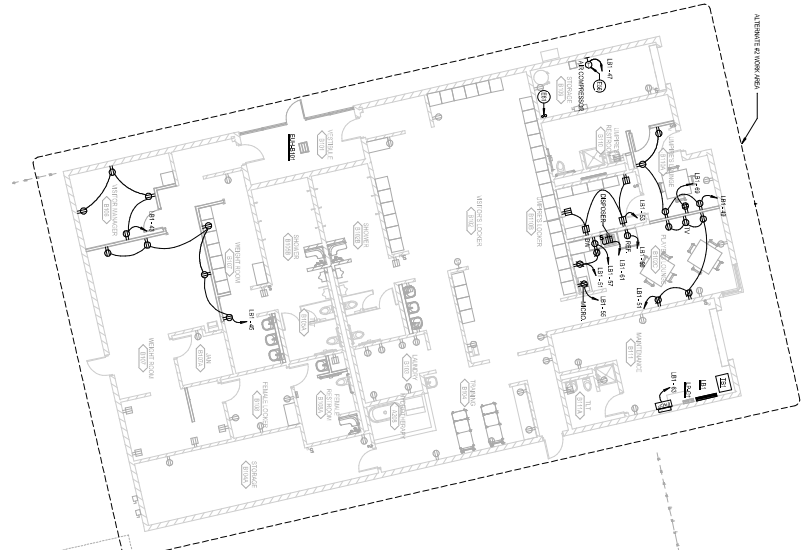
POWER PLAN - AREA B - LEVEL 1 - ALTERNATE #2 SCALE: 1/8" = 1'-0"
