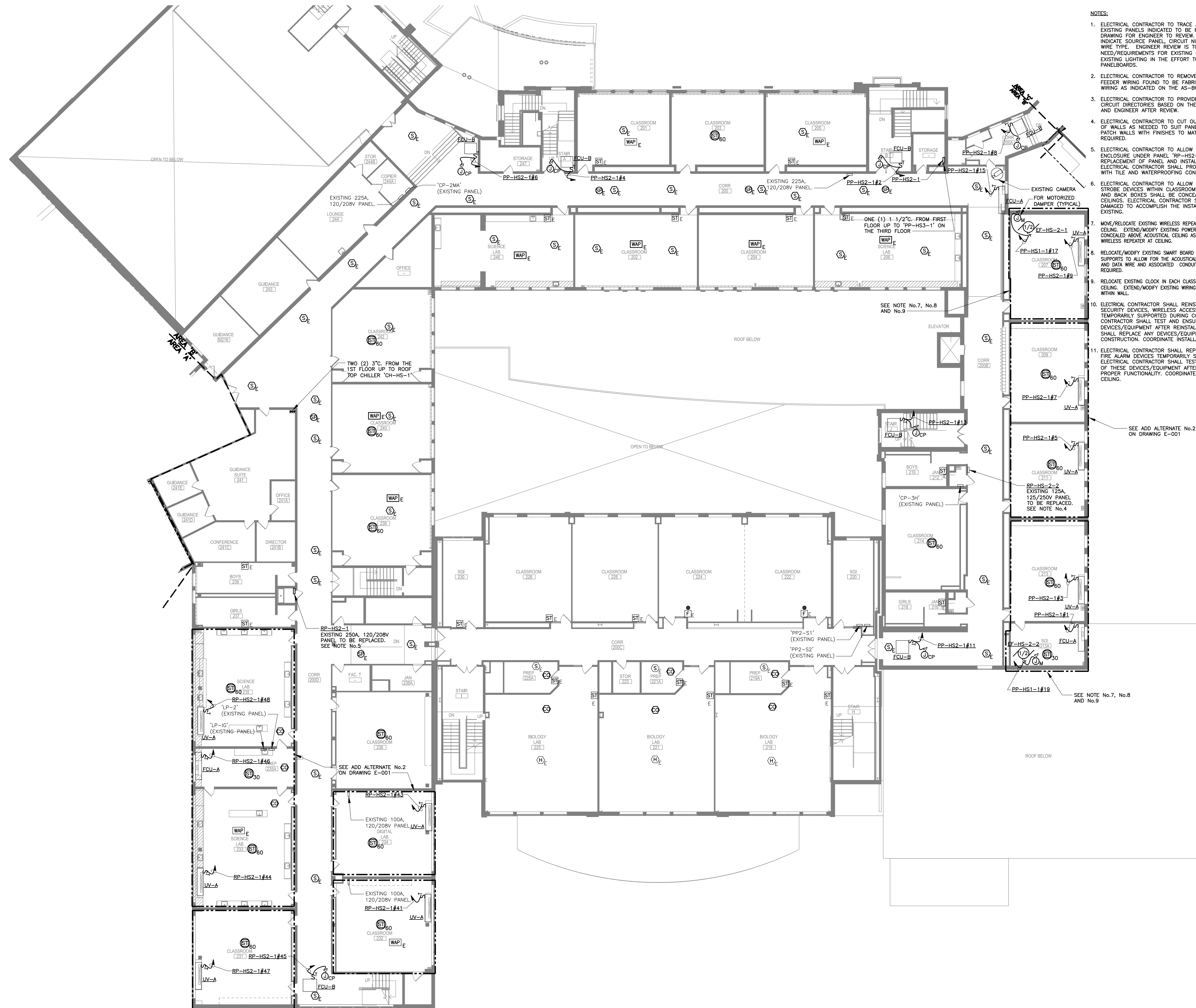
ELECTRICAL PART PLAN - POWER - 2ND FLOOR - AREA B SEE NOTE No.7, No.8 AND No.9 3/32" = 1'-0"
