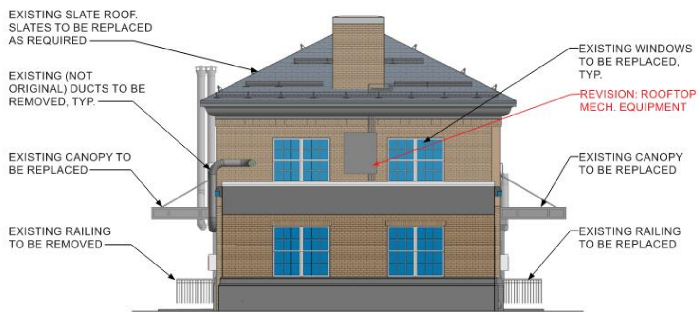
③ EXISTING SOUTH ELEVATION
