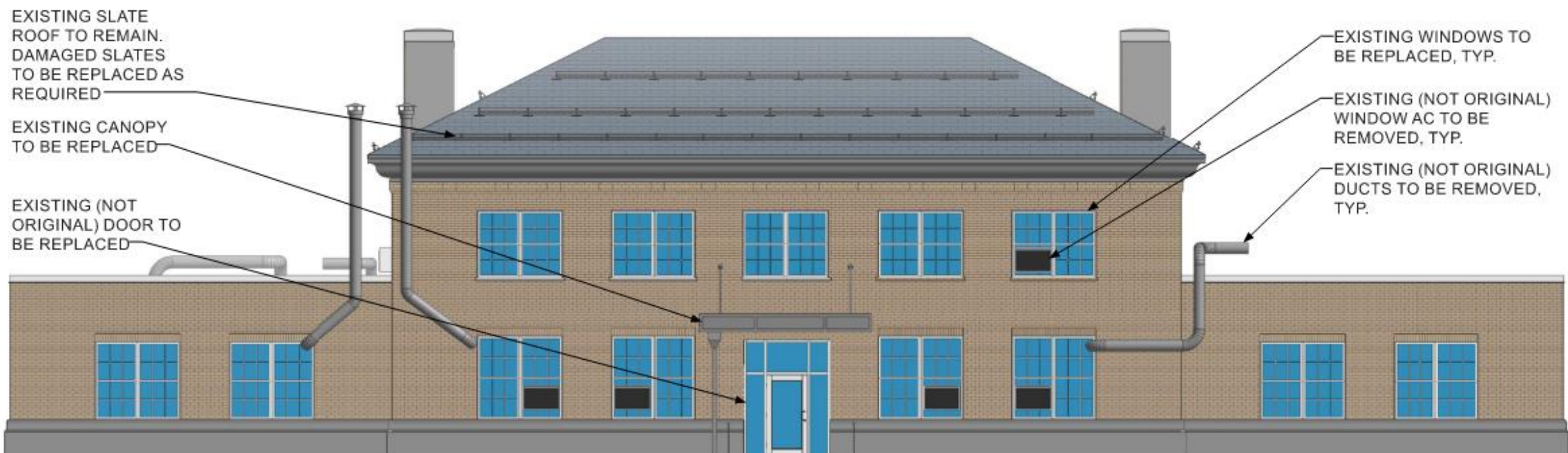
① EXISTING WEST ELEVATION
