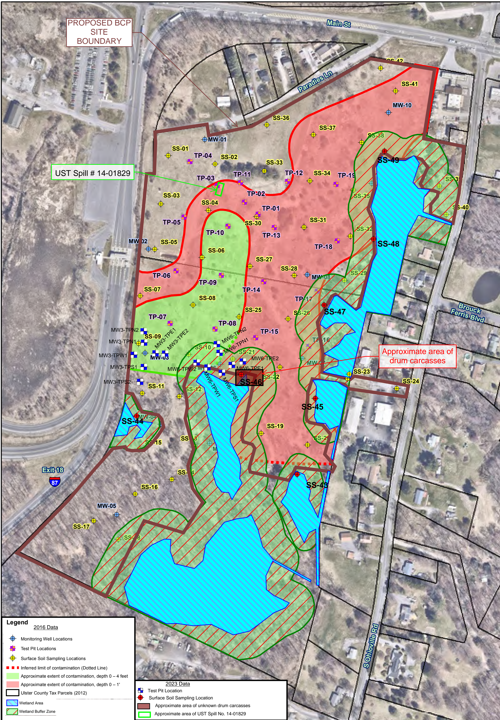
Figure 6: Extent of Contamination in Soils Map and Drum Carcass Area
