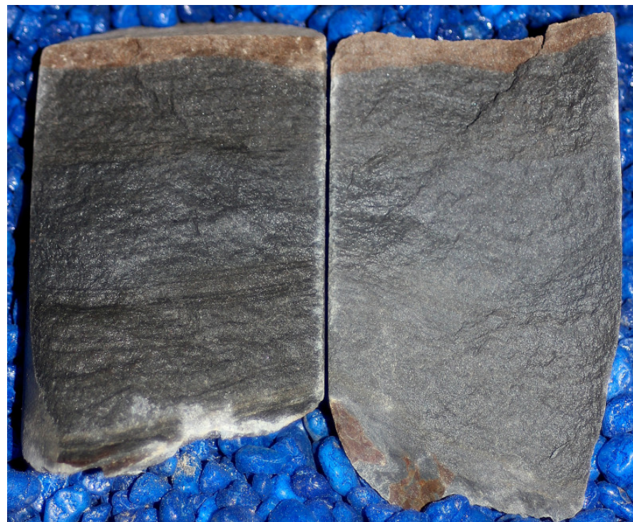
A section of the core, split longitudinally, moistened. Fine laminations are visible in the fine greywacke. At the top end the rock is stained brown, but it is not significantly weathered. The rock had high splitting resistance, and split on a curved surface, which makes the dip of the laminations appear to be shallower than it actually is.
