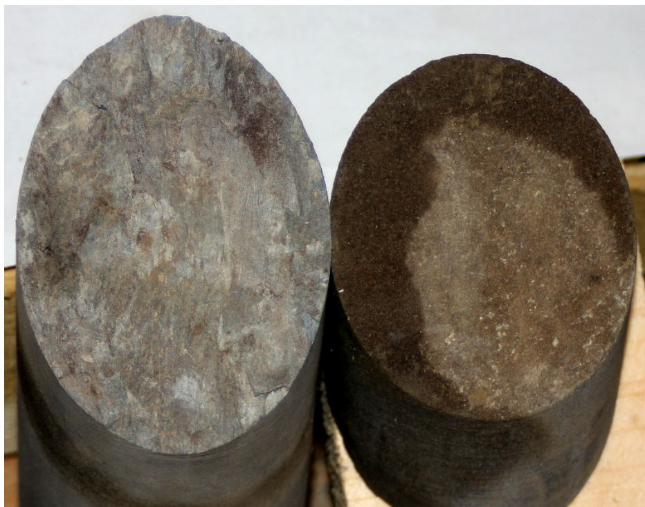
Natural joint surfaces in the core, the left joint in a shale bed and the right joint in greywacke sandstone (partly moistened.)
