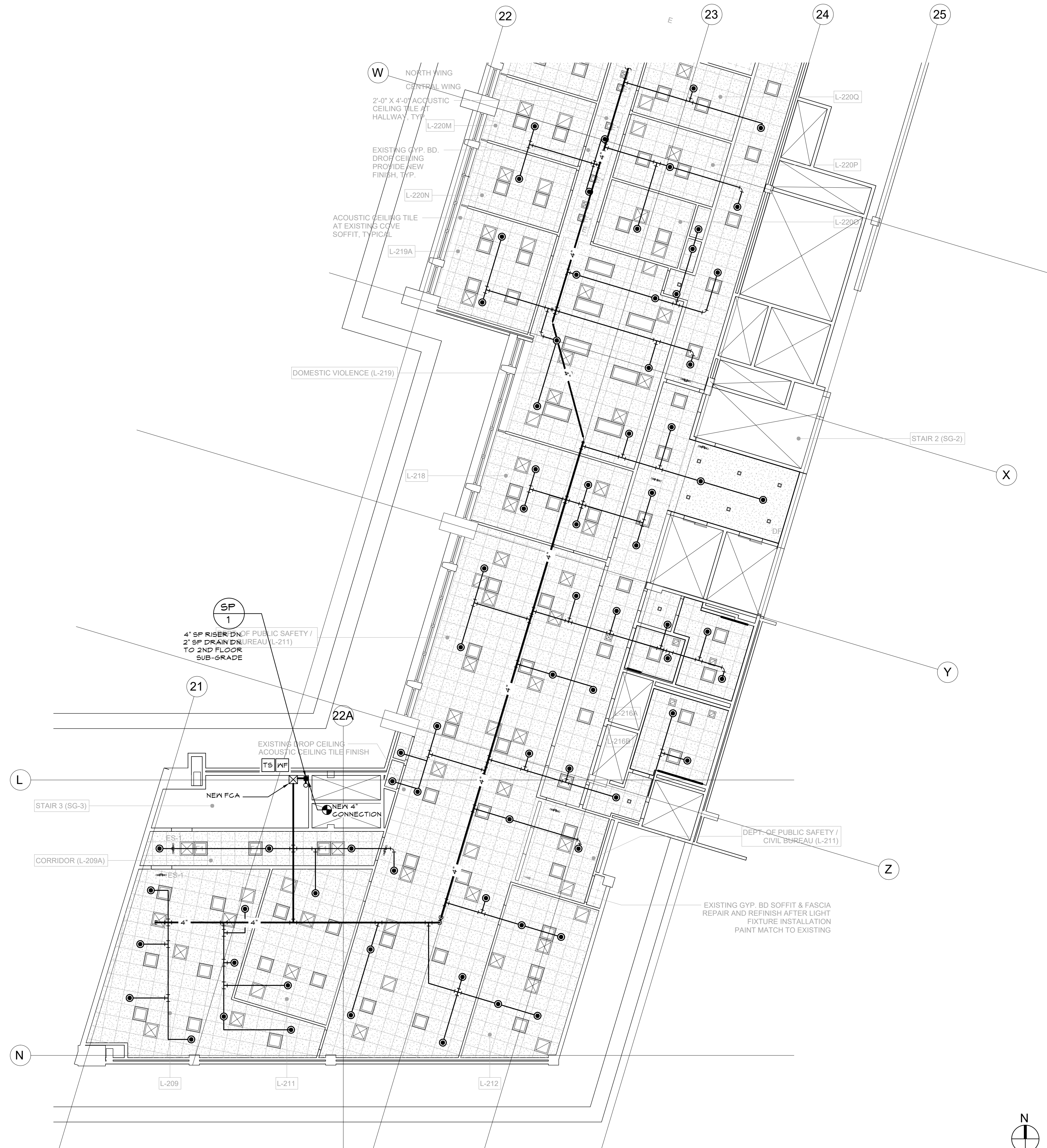
1 SPRINKLER PLAN - 2ND FLOOR CENTRAL WING SP.104 1/8"=1'-0"
