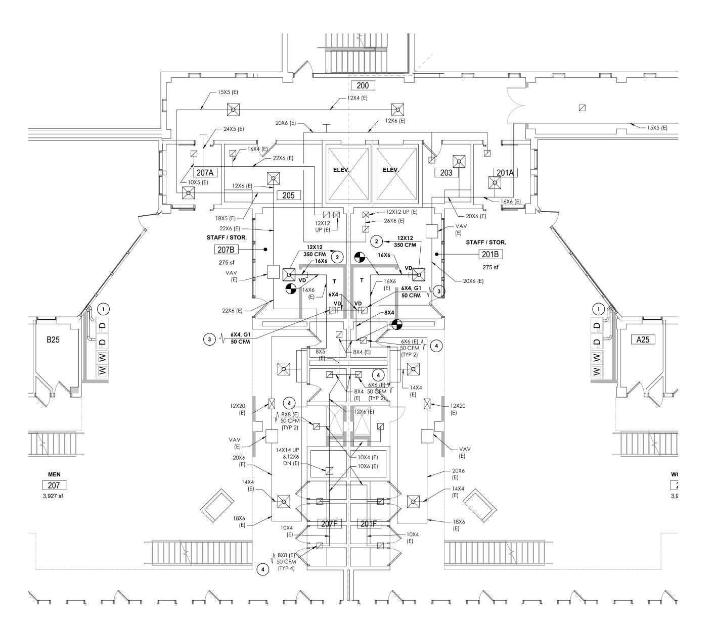
SECOND FLOOR NEW WORK PLAN H202 | SCALE: 1/8" = 1'-0"
