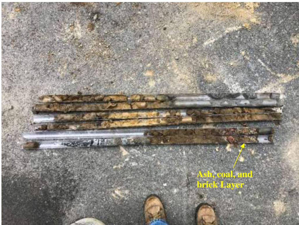
REPRESENTATIVE PHOTOGRAPH OF BORING B-9 SOILS, INCLUDING ASH, COAL, AND BRICK LAYER.
