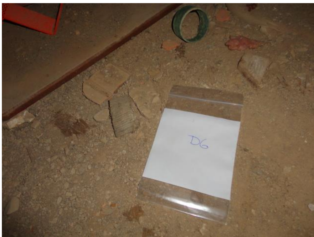
Sample #15 - Debris Location 6 (See Map) - Trace Chrysotile
