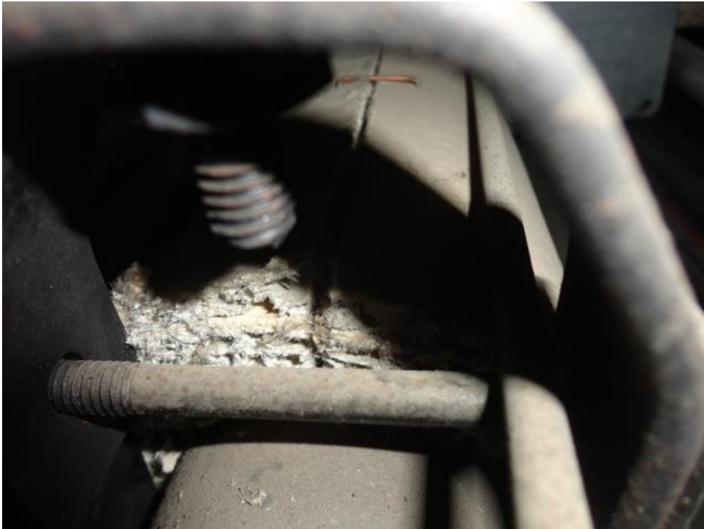
Sample#1 - Air Cell Pipe Insulation - 44.4% Chrysotile
