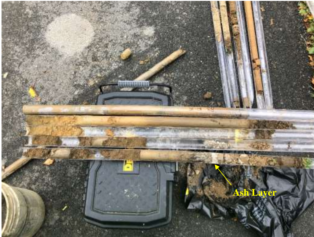
REPRESENTATIVE PHOTOGRAPH OF BORING B-3 SOILS, INCLUDING ASH LAYER.
